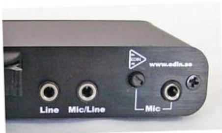
Plug the other end of the patch cord into the "Line" or "Mic/Line" jack on the back of the Univox DLS-50. (They are the same internally although they are labeled differently, so it doesn't matter which one you use.) Note: Don't connect **audio/line outs** to the "Mic" jack, only mic outs, or you risk blowing your Univox DLS-50.
